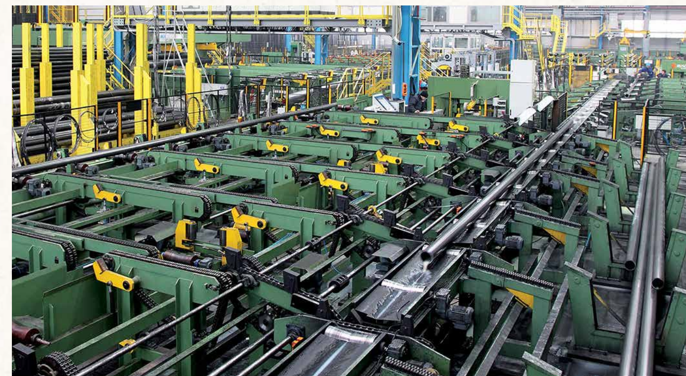
Profiled tubes from hot and cold rolled strip, heat treated and drawn
